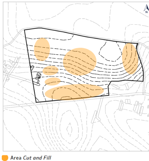
Gambar 3.5.3 Area Cut and Fill
