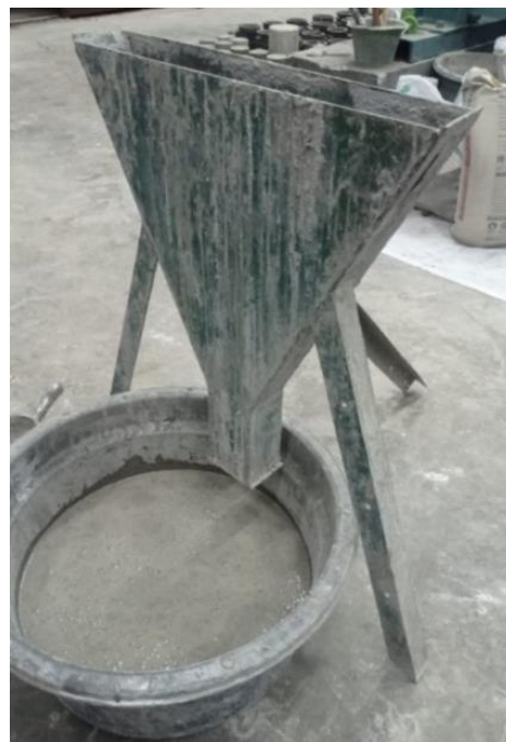
Gambar 3. 3. Alat Uji V-Funnel
