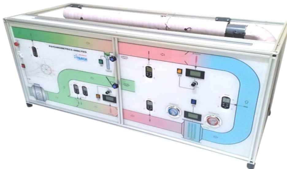
Gambar 3.5 Produk Low-Cost Laboratory Psychrometric Kit (LCLP_Kit)
