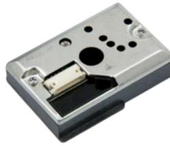
Gambar 3.9 Sensor GP2Y1010AU0F (<https://jk-impex.com/>)
