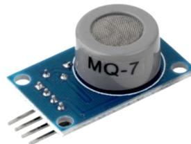
Gambar 3.7 Sensor MQ7 (<https://punoscho.in/>)
