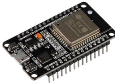
Gambar 3.4 Mikrokontroler ESP32 (<https://techiesms.com/>)
