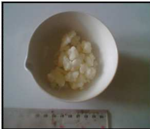
Gambar 3.3 Xerogel hasil proses sol-gel.
