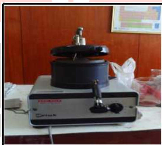
Gambar 3.7 Mesin gerus Karl Kolb scientific technical supplies D-6074 .
