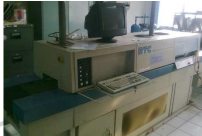
Gambar 3.21 Conveyor Belt Furnace RTC LA-310
