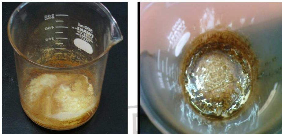
**Gambar 4.1** *Oleil Imidazoline* hasil sintesis *microwave*
