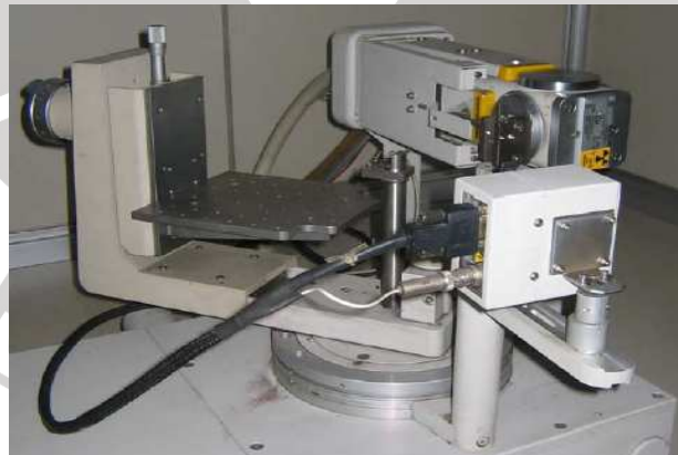
Gambar 3.3 Foto alat XRD Phillips Analytical PW 3710.
