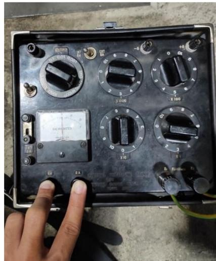
Gambar 3. 7 *Portable wheatstone bridge type 2755*
