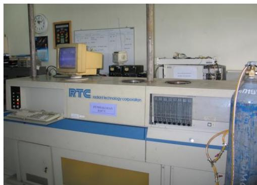
**Gambar 3.24** *Conveyor Belt Furnace* RTC LA-310
